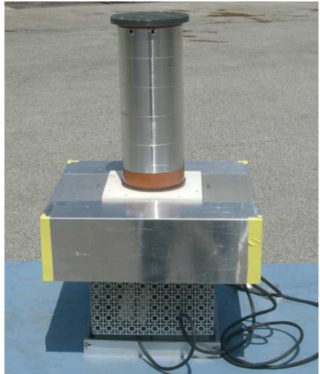
Fig. 1. A detector with shielding (see text) before being mounted on the tower.
