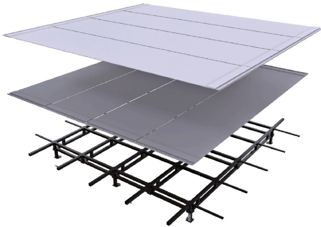
Fig. 32. The TT wall, measuring 7.6 \times 7.6 \text{ m}^2 , assembly on its support frame called a “table”.
