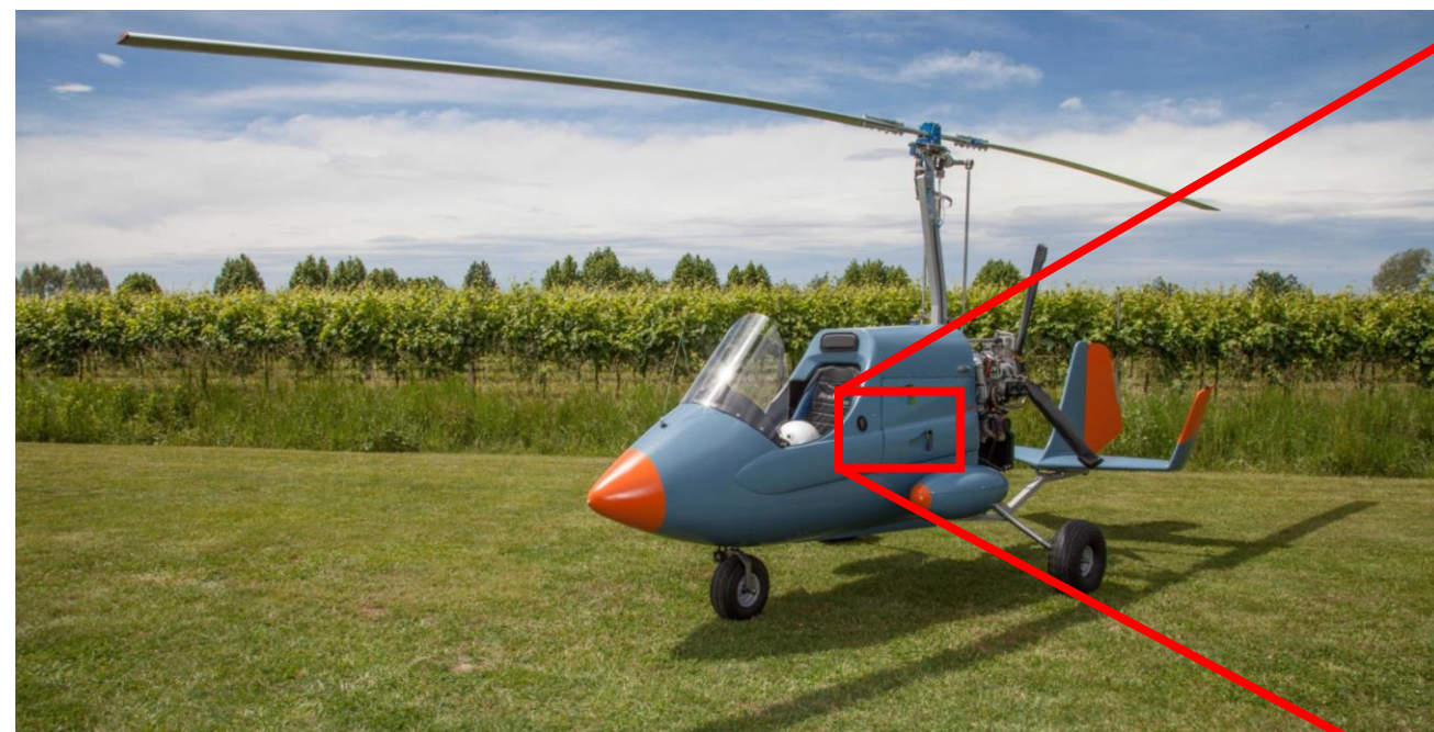
Radgyro: the experimental autogyro devoted to airborne multiparametric measurements
