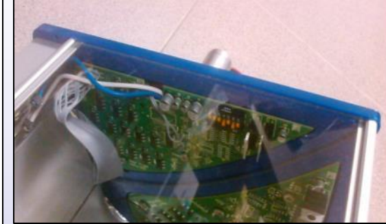
Led Driver PCB mounted on Solar FLight
