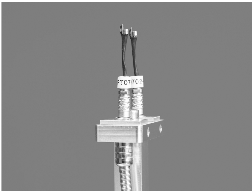
Figure 3.4.1: The hyper-intensimetric system: detail of the twin probes mount specially designed for the Microflow ® kit #133 at the Acoustics Lab of Physics Department-Imamoter, Ferrara University.
