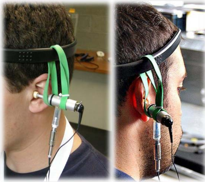
Figure 12. The prototype probe for p-v tympanometry is fitted to the ear canal at normal pressure conditions without sealing the external auditory meatus and having care to align the probe and canal axes.
