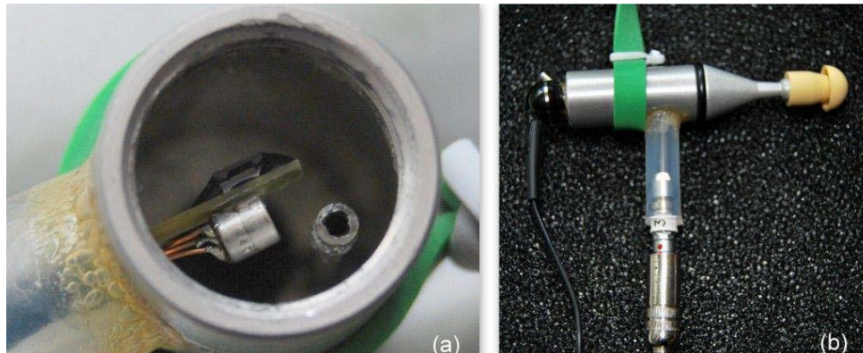
Figure 6. (a) Detail of the p-v sensor inside the prototype probe; (b) Overview of the p-v tympanometric probe.
