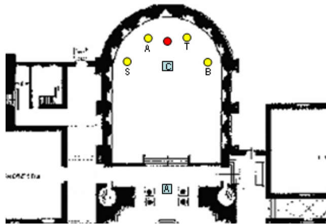
Figure 1: Source-receiver configurations. The yellow spots S, A, T, B indicate the position of the source corresponding to the four sections of the choir; the red spot is the single source position representing the whole choir. The squares represent the positions of the receiver: C is the position of the conductor and A represents the audience.
