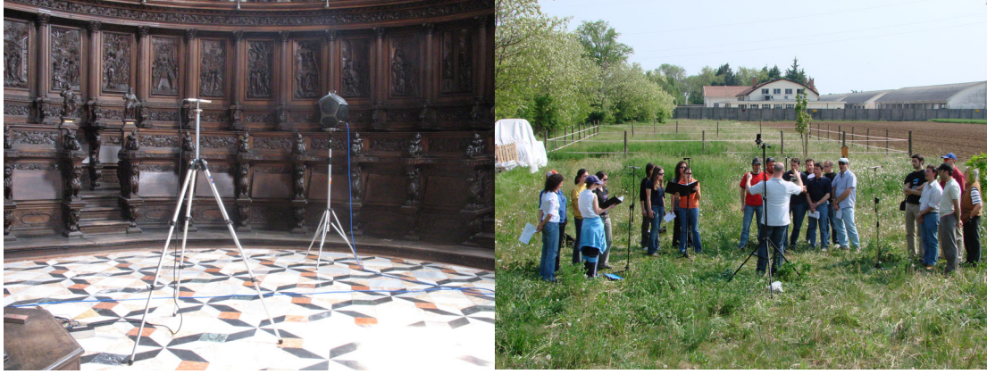
Figure 2: Left: omnidirectional loudspeaker and sound intensity probe in St. George church. Right: recording the choir in an open field.
