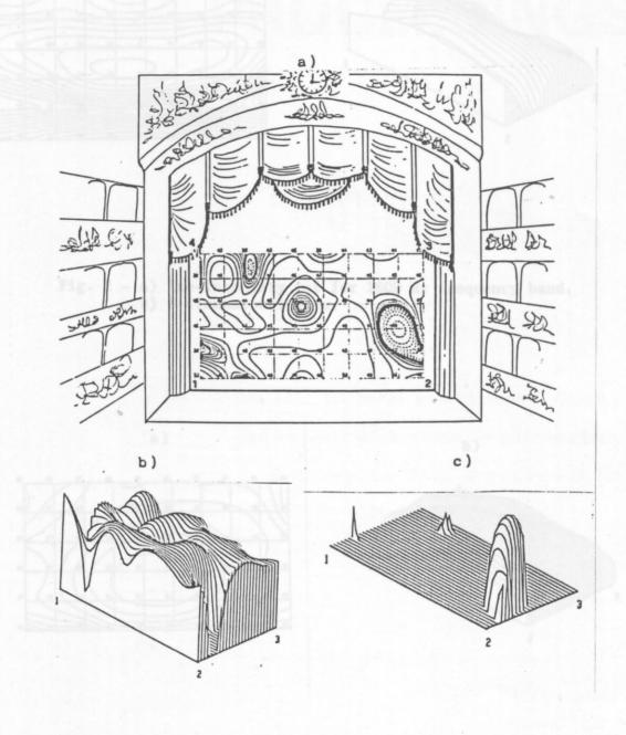
Fig. 1 - a) Iso-intensity map for 50 Hz frequency band.
